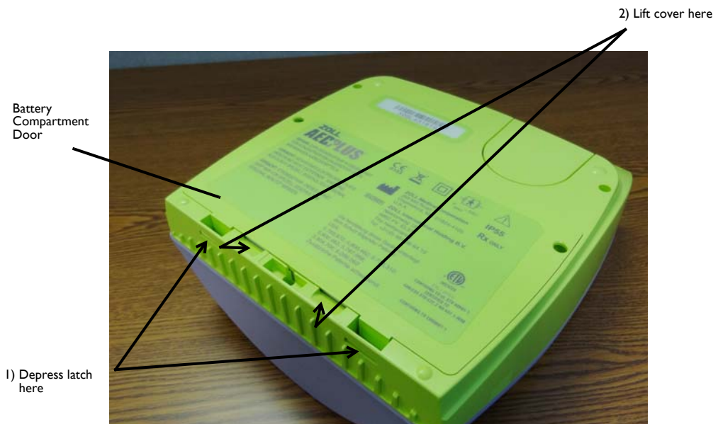
Figure 7: Removing the Battery Compartment Door
