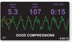
The AED 3 BLS can be easily configured to show the CPR Dashboard<sup>™</sup> only, or both the CPR Dashboard and ECG. Depth and Rate indicators are highlighted in red if the compression rate is too slow and/or the depth is too shallow when in adult rescue mode.
