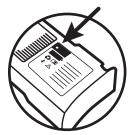
The battery pack's Active Status Indicator ("ASI") is located on the label face of the battery pack and is used to indicate battery pack status. A periodically blinking green LED indicates that the battery pack status is OK and the battery pack is ready for use. Absence of a blinking green LED indicates a battery pack problem or a depleted or missing 9V battery. Refer to the "Checking DDU-120 AED Status" section for information on battery pack LED indications.
