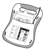
The pad package can then be stored in the pad storage slot in the back of the *DDU-120* AED. After connecting the pads connector to the unit, push the pad package, with the pictures on the package facing up and out, rounded end first, into the pad holder compartment on the back of the AED. When the pad pack is fully inserted, press the pad cable into the groove in the back of the unit to hold it in place and tuck any excess cable behind the pad package.
